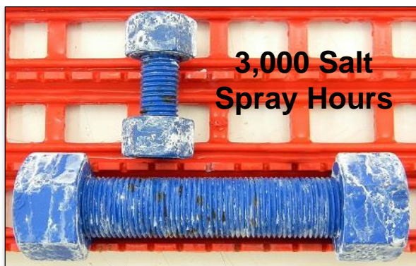
Photos Samples at 3,000 Salt Spray Hours conducted by Assured Testing Services. Coated by Southwestern Plating Company. Bolt Treatment: 0.3-0.5 mil zinc plating with 0.8-1.2 mil of 857G-018
